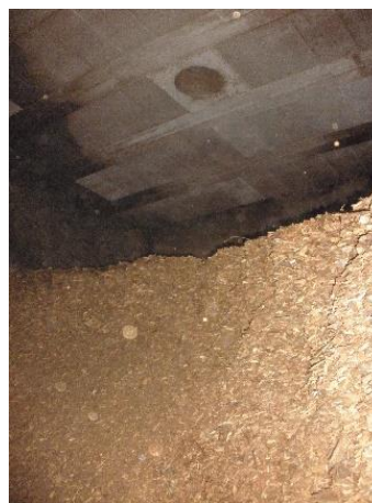
Figure 31: example of rotary silage unloader at the bottom of the silo with extraction screw (left) / example of vertical accumulation of wood showing the not very fluid character of wood chip (right). Source AILE.
