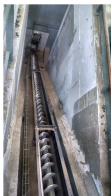
Figure 33 : example of screw conveyor very simple to recommend - source AILE
