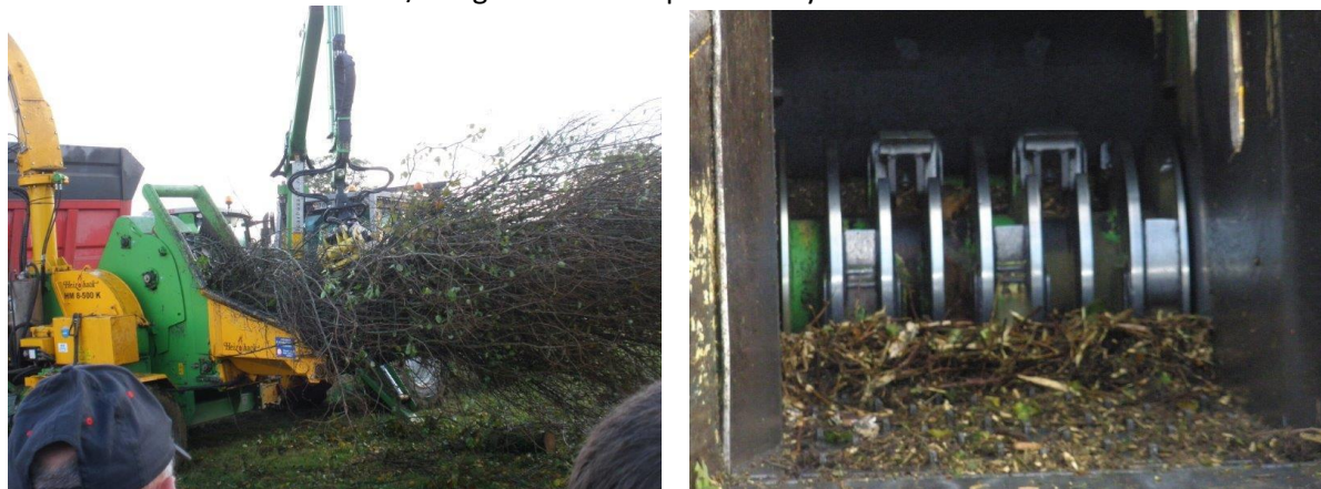
Figure 21: Branches too thin, in leaf = poor yield (clogging) and poor chip quality in combustion. Source: AILE.
