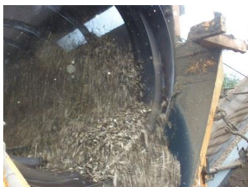
Figure 23 : Trommel screening producing two fractions – source AILE
