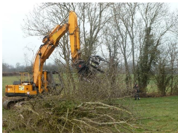
Figure 18: The intervention of an excavator equipped with a harvester head. Sources: Cuma Calvados Innovation and AILE
