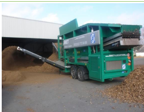
Figure 24: Photo :: Stars screening producing three fractions – source AILE
