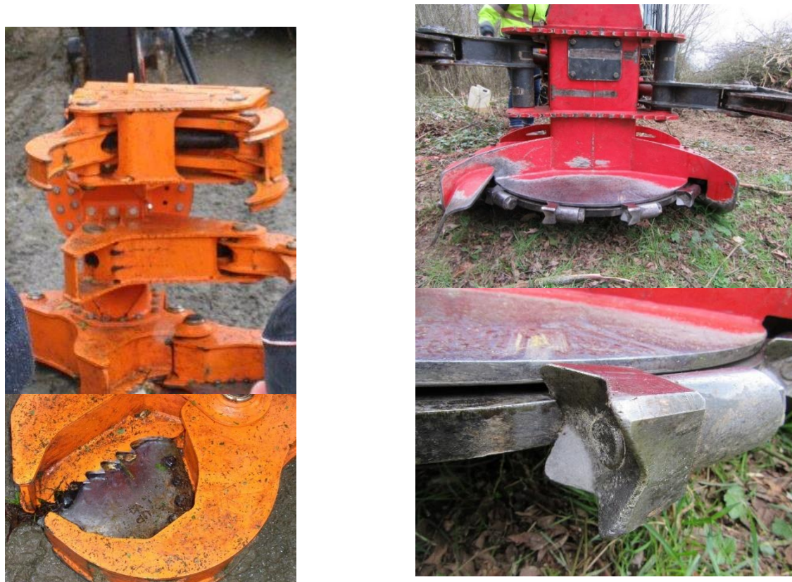
Figure 19: Clamp harvester head (left) and Chain disk harvester head (right). Source: AILE
