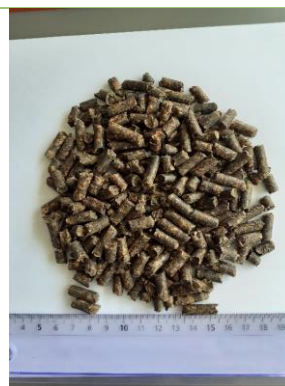
Figure 27: Olive tree pruning pellets fuel [Image source: CERTH / AGROinLOG project] 23
