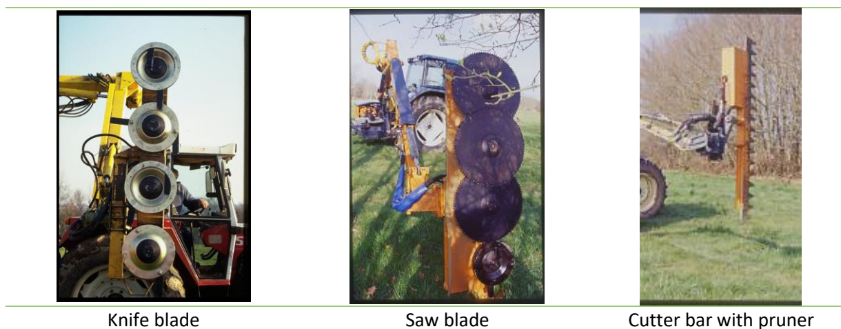
Figure 16: Mechanised lateral tools for hedge. Source: AILE
