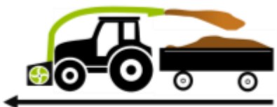
Shredder mounted in front with discharge on agric. trailer
