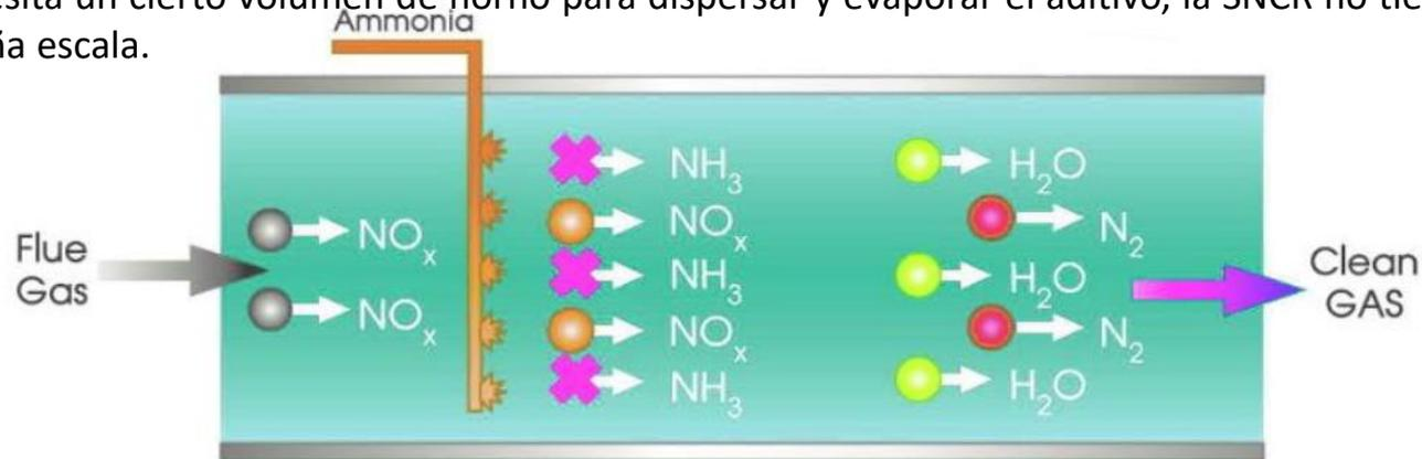
Figure 23: Selective non-catalytic reduction [Image source: IFS<sup>23</sup>]
