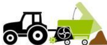
Shredder towed with built-in dump / tilting container
