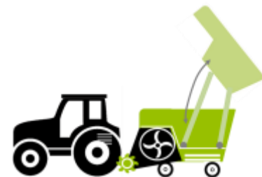
Shredder towed with built-in tilting container discharging on height
