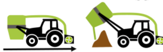
Shredder mounted at rear with discharge on a bin mounted at front lift
