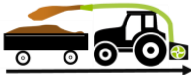
Shredder mounted at rear with discharge on agric. trailer
