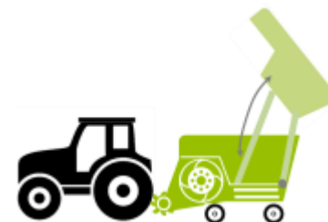
Chipper towed with built-in tilting container discharging on height
