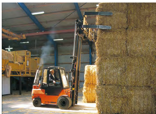
Straw bales are placed in the buffer storage with a forklift truck. The bales must be unloaded and placed within the area marked yellow, so that the crane automatically can collect the bales from the storage.
