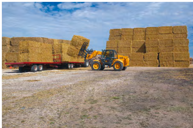
Unloading two bales of straw at once with a telescope loader reducing the workload. PHOTO Torben Skøtt, BioPress.
