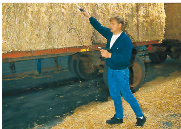
The moisture content in the straw is controlled before the unloading takes place. If the water content is above 25% it is normally rejected.
