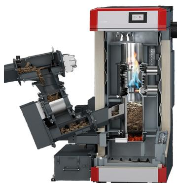
A revolutionary example of state of the art combustion systems with high fuel flexibility are **biomass gasification boilers** that include an updraft gasifier, a gas burner and a hot water boiler. Such systems can achieve almost zero CO and OGC emissions, significantly reduced NO<sub>x</sub> emissions (compared to conventional fixed-bed combustion technologies) and very low particulate matter emissions.
